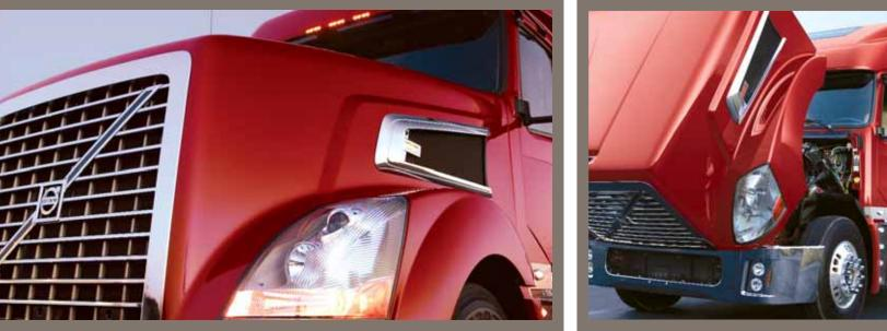
YOU'LL SPEED THROUGH SERVICE CHECKS IN RECORD TIME. Daily service checks on your 880 can be performed easily from the ground. The hood release is mounted on the steering column, which keeps it secure yet easy to reach without having to climb up into the cab. The hood opens a full 60 degrees for complete engine access. Fill sites are on the "cool" side of the engine. Inside the cab, the twopiece engine cover can be removed without taking out the seats or floor mats.
