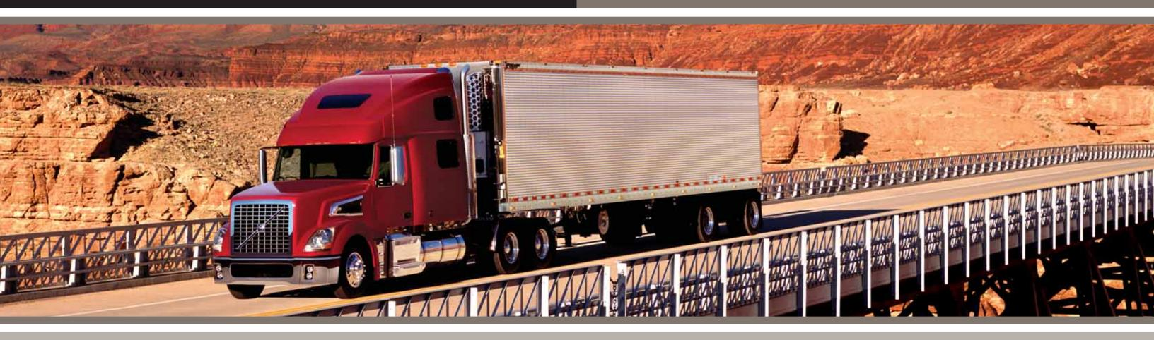
The Volvo VT 880 features rugged suspensions that spare you bumps, bounces and noise. Even Volvo's D16 625 horsepower engine is matched to an innovative Non-Torque-Reactive suspension. This design easily handles the 2,250 lb-ft torque and delivers a more comfortable ride with the added benefit of less component wear. So even with Volvo's 16-liter engine and a full payload, the 880's suspension maximizes the handling and performance of the entire vehicle.
